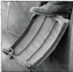
Cockpit door without crowbar brackets, the same type fitted to R6923 A . See also page 13.
